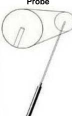
For liquids and gels. Protected from tip to handle by an Inconel sheath. Suitable for general temperature measurement applications. Measurement range: - 196°C to 800°C (-320°F to 1472°F)
