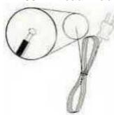
Included with APPA50 series. General purpose applications. Teflon tape insulation. Not suitable for liquid immersion. Measurement range: -40°C to 204°C (-40°F to 399°F)
